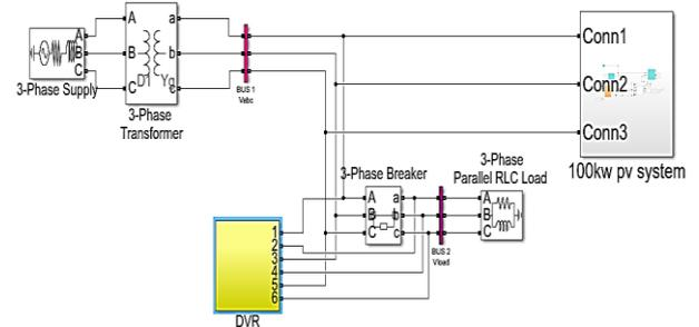
**Figure 6.** The proposed PV integrated system with DVR
