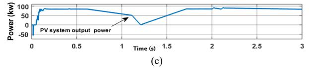
Figure 10. Effect of temperature and irradiance on PV system output: (a) Irradiance; (b) Temperature; (c) PV power output
