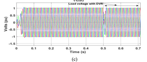
Figure 11. The proposed DVR controller performance in the presence of fluctuant PV power output: (a) PV output voltage; (b) Compensated voltage using the proposed DVR; (c) The voltage profile at the PCC
