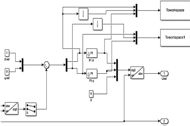
Figure 8. Exporting inputs and outputs datasets from the conventional PI controller.
